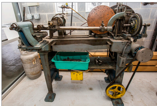
Figure 16 Image of an Augenstein copy and reducing machine
