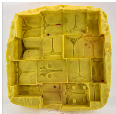
Figure 18 Two-part RTV rubber mold "dummy die" of T-shanks
