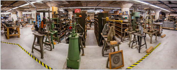
Figure 23 Screw presses set up to create work cells and shelves of old die sets
