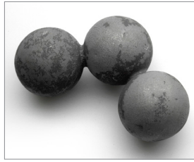
Figure 35 Module of three granules for creating a chaotic structure in Object #5: sterling silver, 3.2 mm x 5.0 mm x 8.6 mm (.126 in. x .197 in. x .339 in.)
