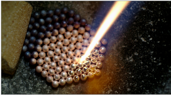
Figure 27 Object #3 in progress; the pre-granulated triangle “grows” further.
