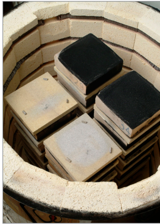
Figure 20 Filled crucibles are closed and put into the kiln.
