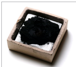
Figure 19 Filled ceramic tile is covered with a piece of thin paper and charcoal powder.
