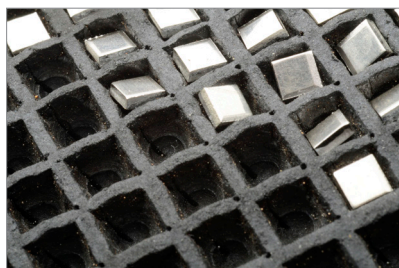
Figure 17 Ceramic tile for granule production: sterling silver coupons, 3.7 mm x 3.7 mm x 1.25 mm (.146 in. x .146 in. x .049 in.)
