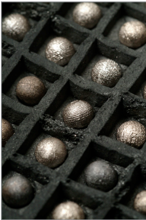
Figure 24 Granules (sterling silver, 3.2 mm/.126 in.) are coarse due to the slow solidification process.
