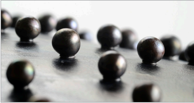
Figure 2 The neck between granule and surface: sterling silver base, sheet 0.8 mm (20 ga), fine silver granule 2 mm (.078 in.)
