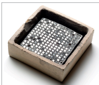
Figure 18 Filled ceramic tile is placed on the bottom of a flat refractory crucible.
