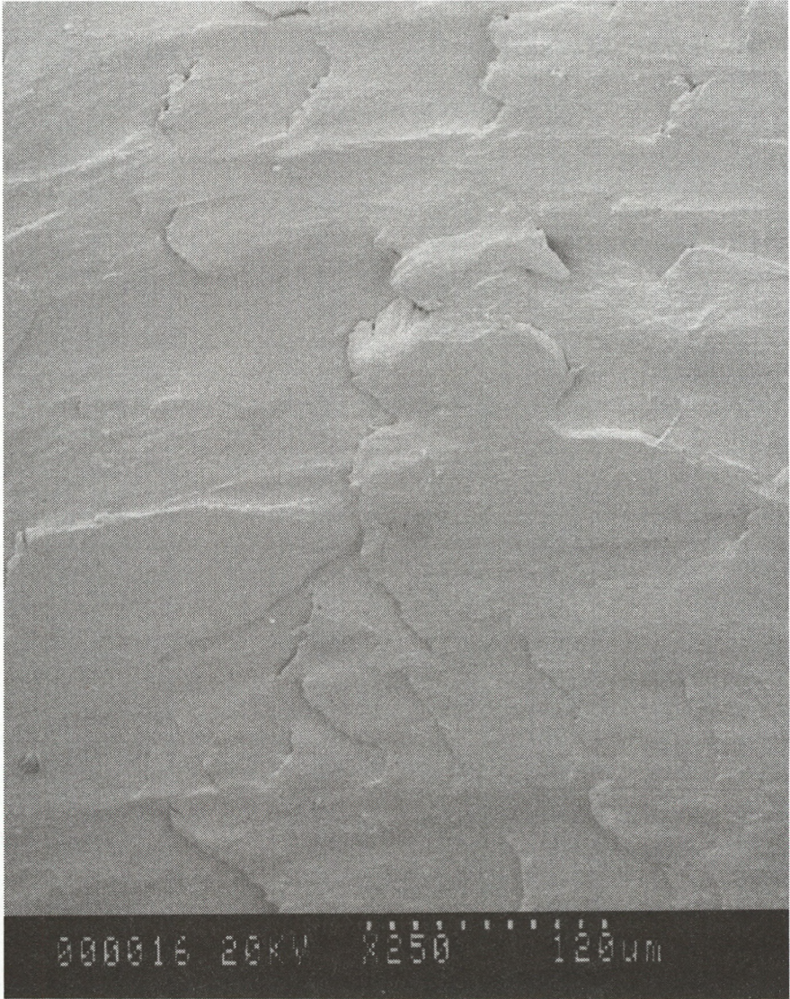
Figure 9: SEM image of 95%Pt HTA first dilled hole
