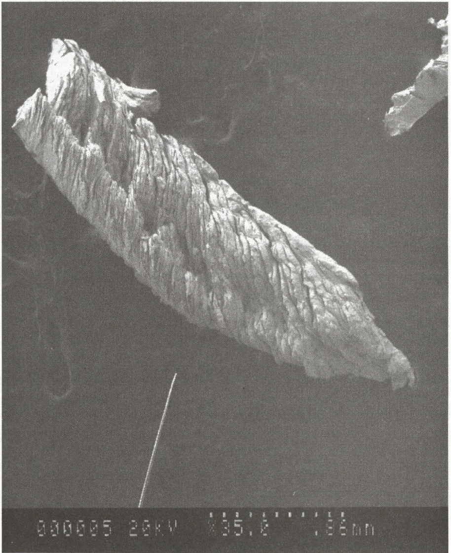
Figure 12: 95%Pt-5%Ru drill chip; note rough surface
