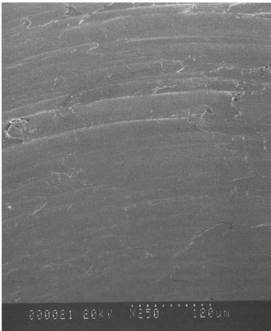
Figure10: SEM image of 95%Pt-5%HTA last drilled hole
