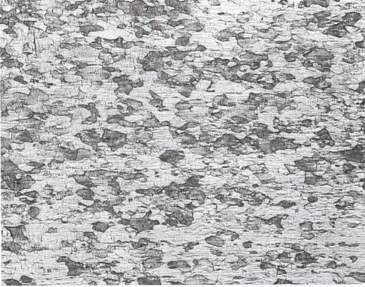
Figure 1 The longitudinal (parallel to the tube axis and tube radius) grain structure of the Pt-4.8Ru alloy tube is shown. The structure is elongated in the direction of tube drawing. The grain size is an ASTM #6. The hardness is VHN100 184. Magnification is 100x.
