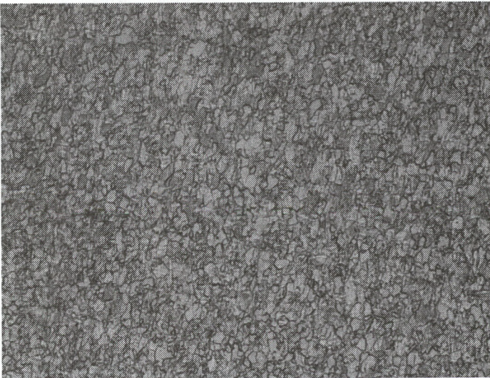
Figure 2 The transverse (perpendicular to the tube axis) grain structure of the Pt-4.8Ru alloy tube is shown. The grain size is an ASTM #7. Magnification is 100x.
