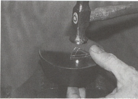
Figure 7e. Hammer welds to match individual wire height.
