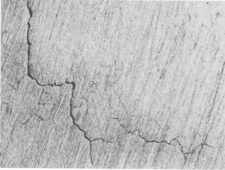
Figure 2. Surface of failed 18ct MBG workpiece. Mag x 30.
