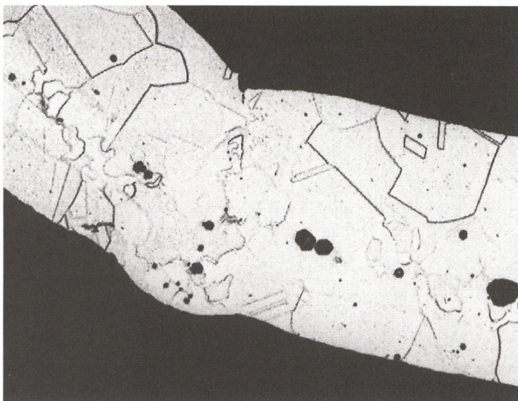
Figure 17. Excess solder fillet in a 14ct link. Mag x 320.
