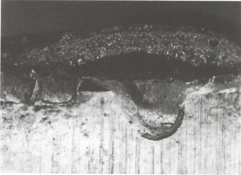
Figure 9. Photograph of the 1T bend of the brazed bevel joint of the 0.030 inch thick, Pt-4.8Ru strip at 15x.
