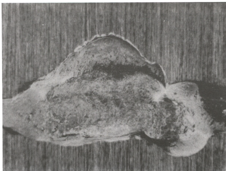
Figure 5. Photograph of the brazed bevel joint of the 0.030 inch thick, Pt-4.8Ru alloy at 15x.
