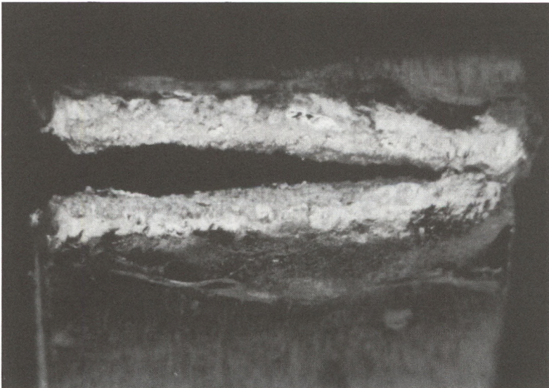
Figure 24. Photograph of the 1T bend of the brazed butt joint of the 0.030 inch thick, Pt-4.8Ru alloy casting at 10x.
