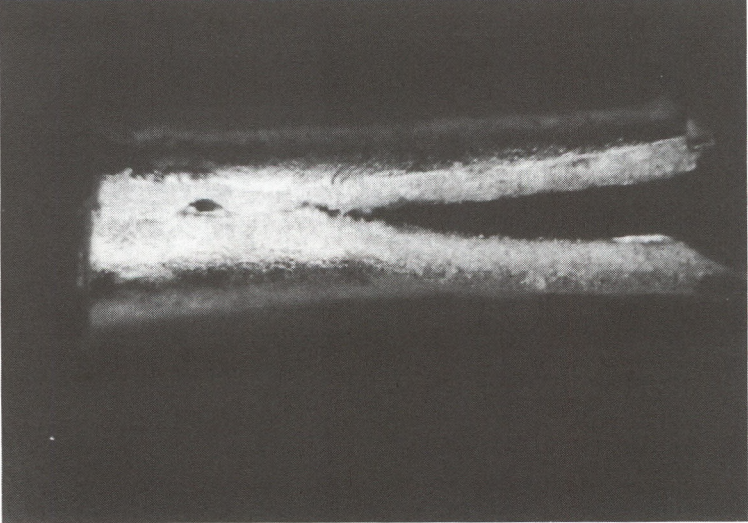
Figure 43. Photograph of the 1T bends of the brazed butt joint of the 0.030 inch thick, 18kt gold strip at 10x.
