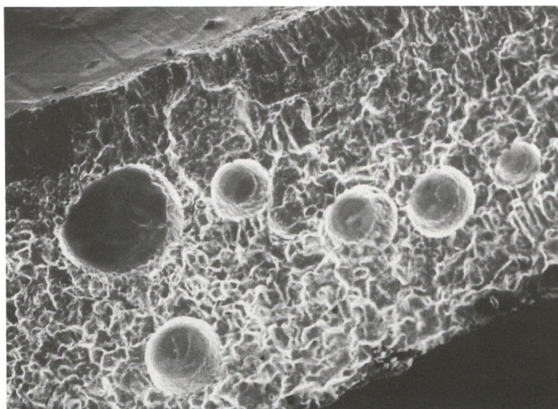
Figure 16. Scanning-electron-micrograph shows the fracture surface of the 1T bends from the brazed butt joint using 1700 Pt solder on the 0.030 inch thick, Pt-4.8Ru alloy strip at 100x.
